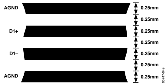
Figure 61. Arrangement of Signal Tracks
